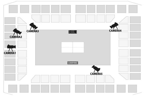
Camera 1: most used camera which shall provide the main wide shot of the game. The camera shall be located on a scaffold (5m high) and positioned in the centre behind the table.
